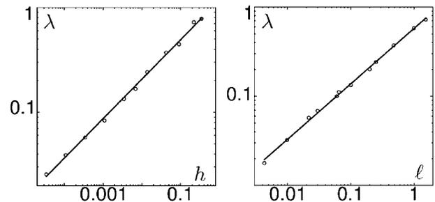
FIG. 3. Numerical check of scaling law  $\lambda \sim h^{2/5}\ell^{3/5}$ : smallest wavelength  $\lambda$  in the cascade versus plate thickness  $h$  (left panel) and metric typical length  $\ell$  (right panel) for the family of metric perturbations  $g_\ell(y) = 1/(1 + y/\ell)$ . Thick lines are best power-law fits, yielding exponents 0.38 and 0.62, respectively.
