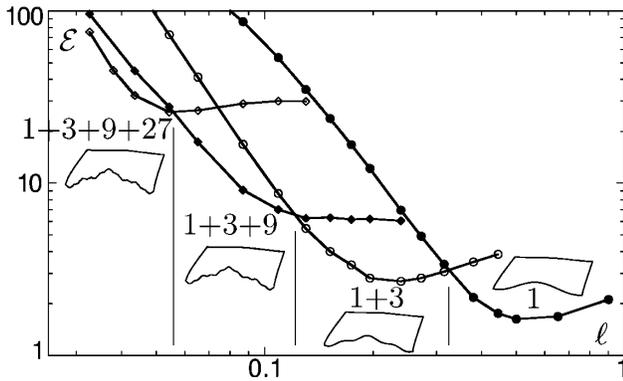
FIG. 4. Total elastic energy of solutions with one to four generations of wrinkles for the one-parameter family of metrics  $g_\ell(y) = 1/(1 + y/\ell)$ . Unit of energy is the bending modulus [i.e., the prefactor of the bending energy in Eq. (2)]. Bifurcations occur while all branches remain close to embeddings: they are selected by minimization of bending energy.
