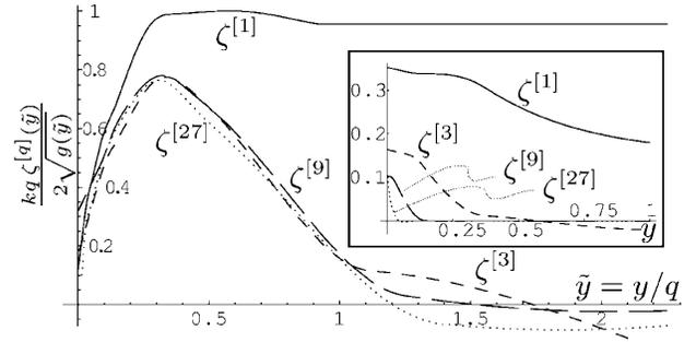
FIG. 2. Fourier components  $\zeta^{[q]}(y)$  ( $q = 1, 3, 9, 27$ ) of the deflection for a numerical self-similar solution with four generations (inset) and their collapse using transform (5).  $\zeta^{[1]}(y)$  need not collapse away from the stretched edge (i.e., large  $y$ ). Same parameters as in Fig. 1, except for  $h = 2.9 \times 10^{-4}$ .
