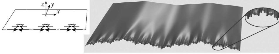
FIG. 1. An elastic plate buckles into a self-similar pattern due to residual strains near the edge (inset). Numerical solution for thickness  $h = 2.9 \times 10^{-5}$ , width 1, metric perturbation  $g(y) = 1/(1 + y/\ell)$ ,  $\ell = 0.008$ , yielding wavelength  $2\pi/k = 0.54$ .
